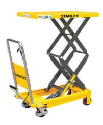
The Stanley Table Lifter 350kg has a double scissor mechanism. This enables it to lift loads up to height of 1,3m without compromising on maximum load capacity. All Stanley lifting tables are raised with a foot pedal and can be proportionally lowered with a hand lever. Lockable rear casters insure a firm working surface.
