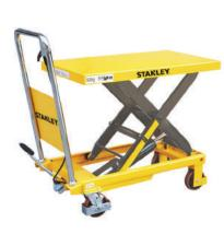
The Stanley Table Lifter 300kg has a scissor lifting mechanism. This enables it to lift loads up to height of 0,9m without compromising on maximum load capacity. All Stanley lifting tables are raised with a foot pedal and can be proportionally lowered with a hand lever. Lockable rear casters insure a firm working surface.
