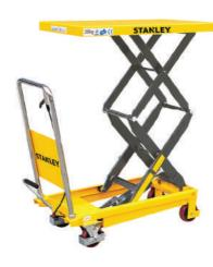
The Stanley Table Lifter 800kg has a heavy duty double scissor mechanism. This enables it to lift loads up to height of 1,5m without compromising on maximum load capacity. All Stanley lifting tables are raised with a foot pedal and can be proportionally lowered with a hand lever. Lockable rear casters insure a firm working surface.
