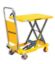
The Stanley Table Lifter 150kg has a scissor lifting mechanism. This enables it to lift loads up to height of 0,9m without compromising on maximum load capacity. All Stanley lifting tables are raised with a foot pedal and can be proportionally lowered with a hand lever. Lockable rear casters insure a firm working surface.
