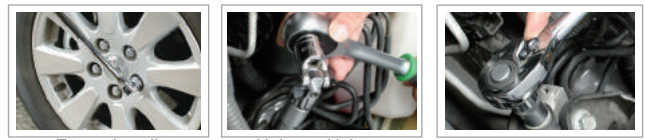
F type handle Universal joint Teeth reverse flat ratchet handle
