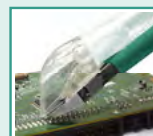
For cutting and control IC pin ends
