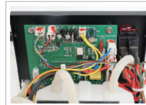
All in 1 PCB Metal screws fixed.
