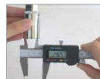
Inside dimension measurement
