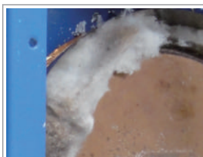
Aluminosilicate heat preservation material
