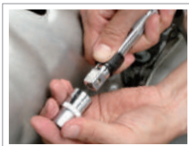
Extension bar with quick release
