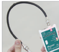
BNC cable test
