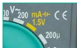
1.5V Battery Test
