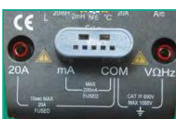
Transistor hFE test
