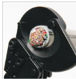
Cutting telecom cable up to 600MCM(300mm 2 )
