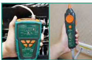
Verify LAN/ telephone cable condition
